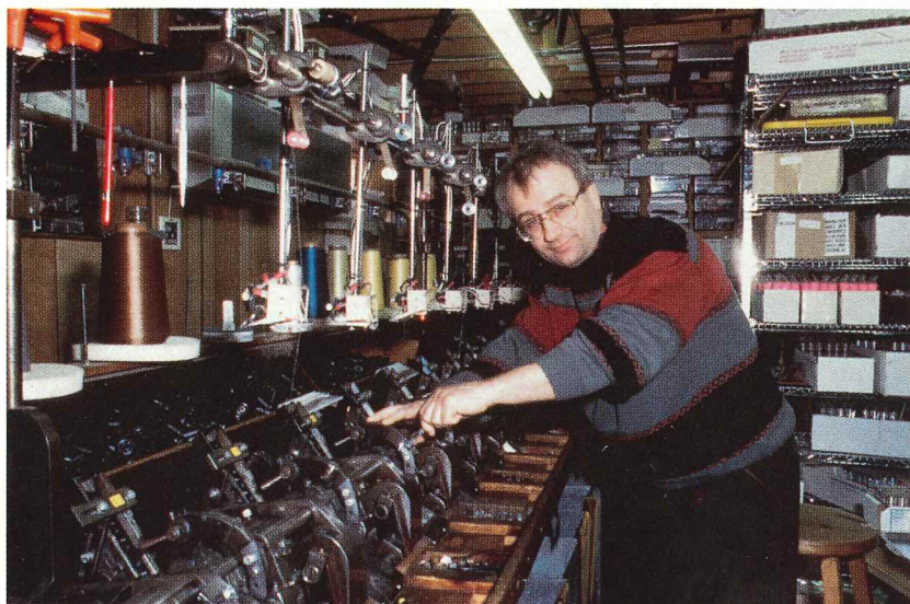
UNI Products owner Jean-Guy Côté adjusts one of the company's spooling machines.
